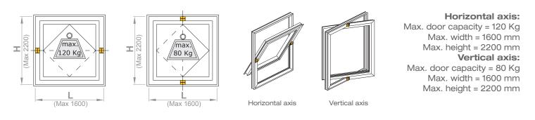
Capacity has been increased up to 120 Kg for the horizontal axis and up to 80 Kg for the vertical axis.
